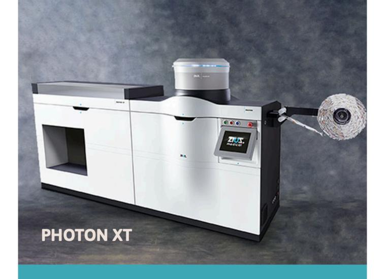
The Photon checks 13 different parameters such as shape, size and colour thus greatly reducing DAA packing errors – it also has the same low error rate as the IRIS of 1.33 sachets per million.
